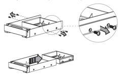
Step 4 Once the installation is completed, insert the tray back and fix it firmly in the proper place.
