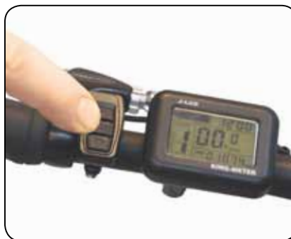
Fig. 9.2 Hold Down “MODE” Button for 2 Seconds
