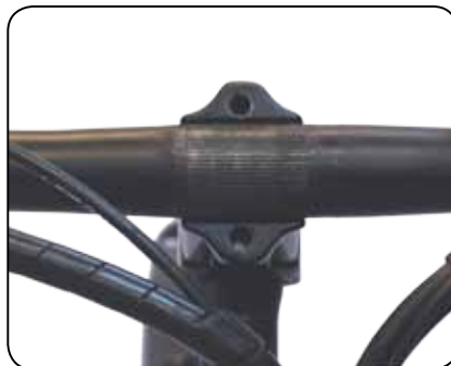
Fig. 1.3 Handlebar Stem With Handlebar Inserted
