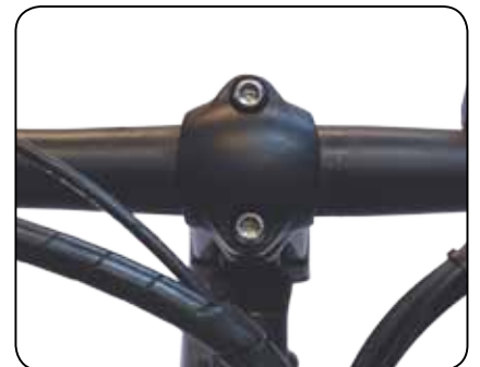
Fig. 1.4. Handlebar Faceplate With Tightened Bolts
