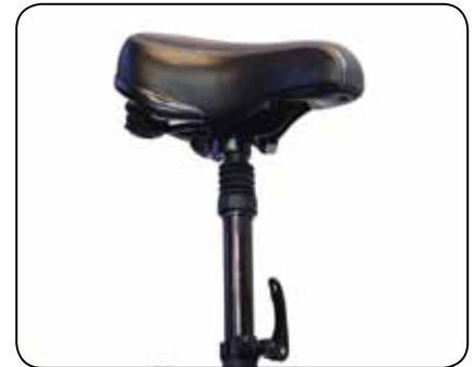
Fig. 4.3 Seat Post Inserted Correctly, Past “Minimum Insert Line”
