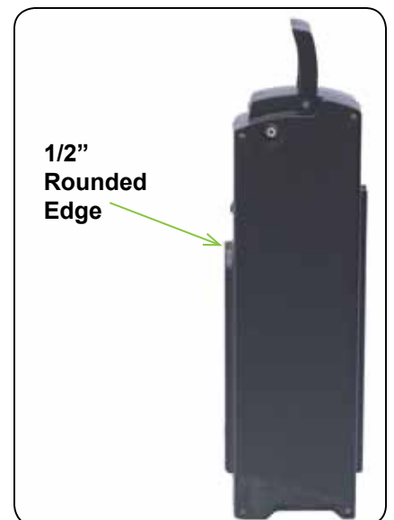
Fig. 6.2 Battery - 1/2" Rounded Edge Towards Seat Post
