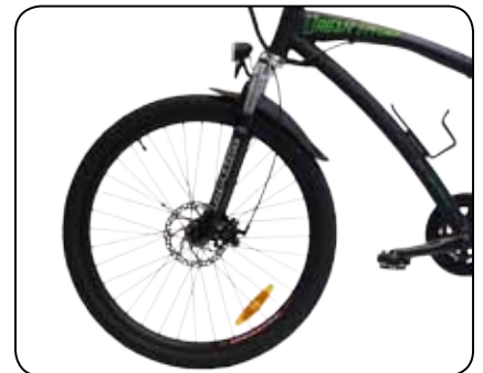
Fig. 2.7 Forks Secured Onto Front Wheel
