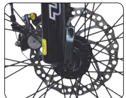
Fig. 2.5 Quick Release Lever In Closed Position
