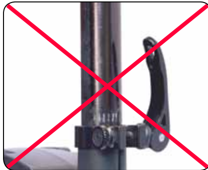
Fig. 4.2 Incorrectly Installed Seat Post
