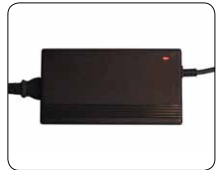
Fig. 7.5 Battery Charging - Red LED
