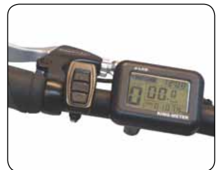
Fig. 11.3 King Meter® Display, Set ASSIST to “0” While Programming
