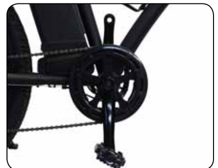
Fig. 3.2 Crank Arm, Right Pedal Inserted
