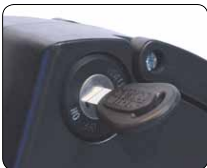
Fig. 8.1 Battery Key - ON
