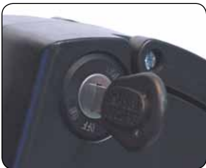
Fig. 7.1 Battery Key - OFF
