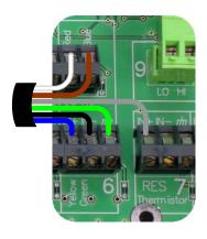
In DeltaLINK<sup>2</sup> configure channel 6 as type **SM300** and channel 7 as a type **SM300 Temperature** sensor.
