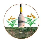
Note: The SM300 is not suitable for soil surface temperature measurements. For soil temperature near the surface dig a trench and install horizontally as shown below. Cover both SM300 and the first 30cm of cable with at least 5cm of soil.
