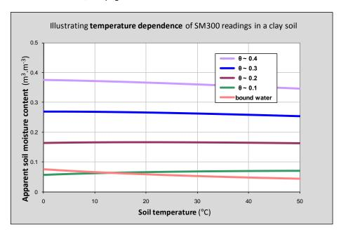
Note: ice has a quite different refractive index from water, so SM300 soil moisture readings cannot be interpreted reliably when inserted into soil below 0°C.
