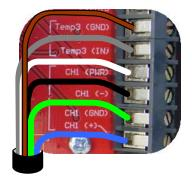
Using the DeltaLINK<sup>1</sup> logger software, configure channel 1 or 2 as sensor type **SM300** and channel 3 or 4 as an **SM300 Temperature** sensor.
