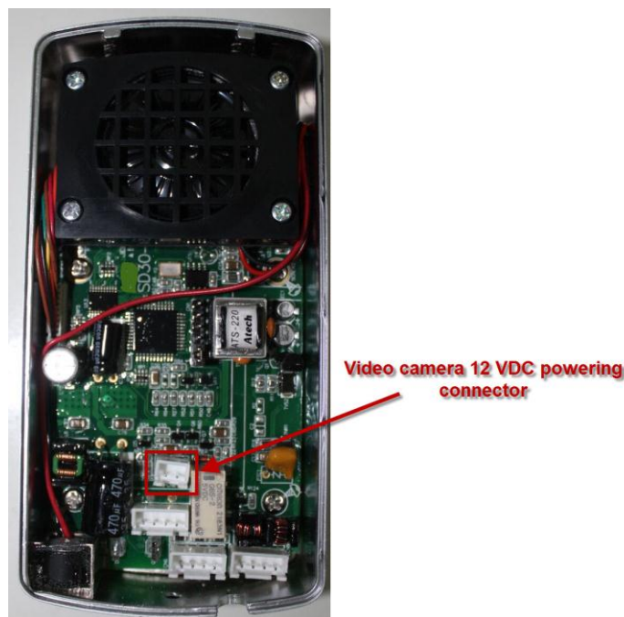
Figure 6-8 The SD-30X External Video Camera powering connector
