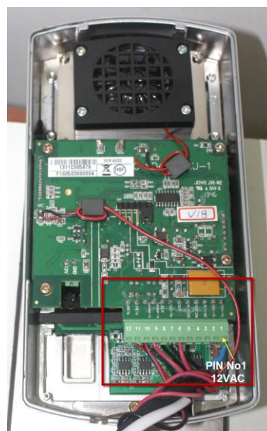
Figure 6-4 The SD-40X Model Door Phone wires connector
