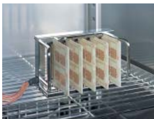
SIR test coupon type IPC-B-24 and test board rack type A (optional)
