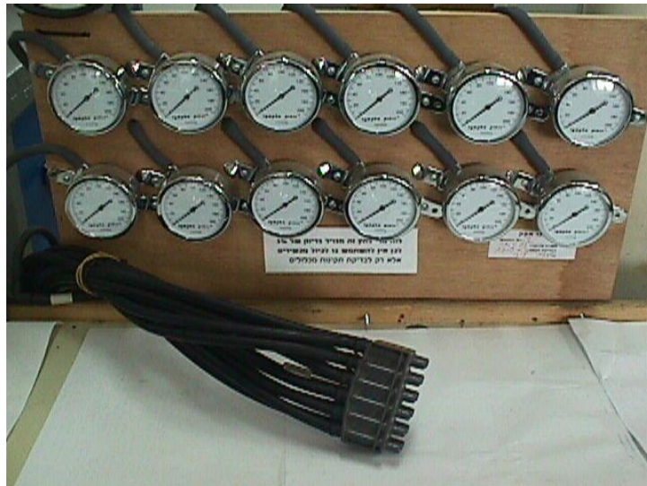
Figure 7.1 - Testing Set (12 Pressure-gauge Board and Hose Bundle)
