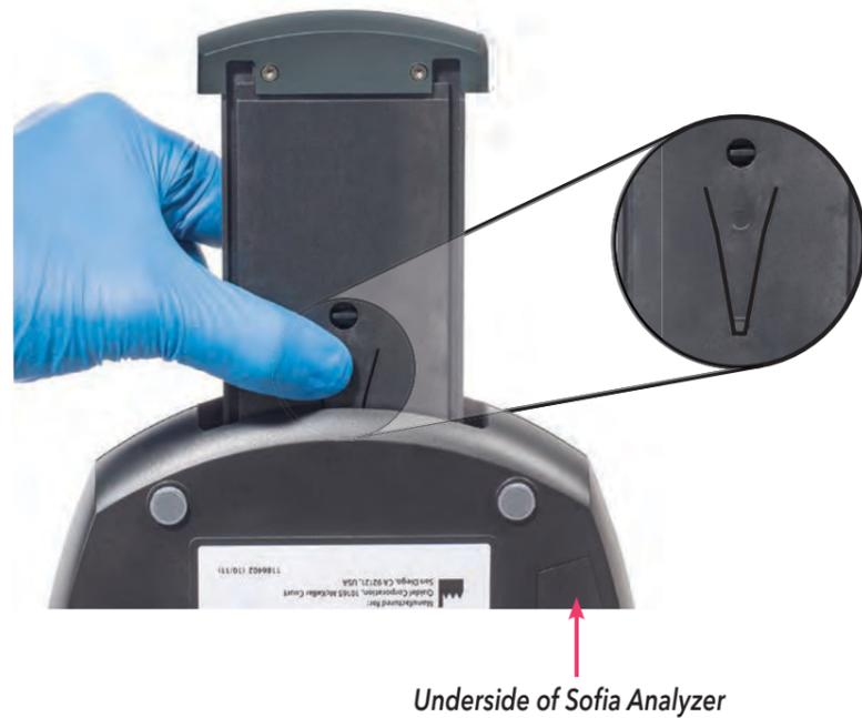
Use a soft cloth with 70% alcohol or 0.6% bleach solution to clean the Cassette drawer only. **Do NOT** clean the interior of the analyzer. **Do NOT** submerge drawer in cleaning solution.
