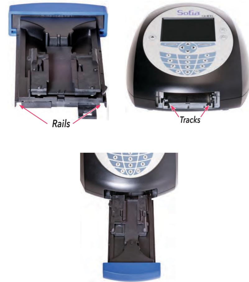
Gently slide the drawer until it is latched closed. If resistance is met or the drawer does not slide easily, check the alignment of the rails in the track.
