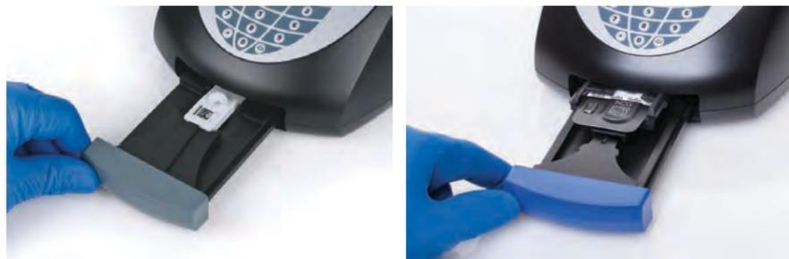
Upon closing the drawer, the analyzer will start automatically and display the progress on the screen.
