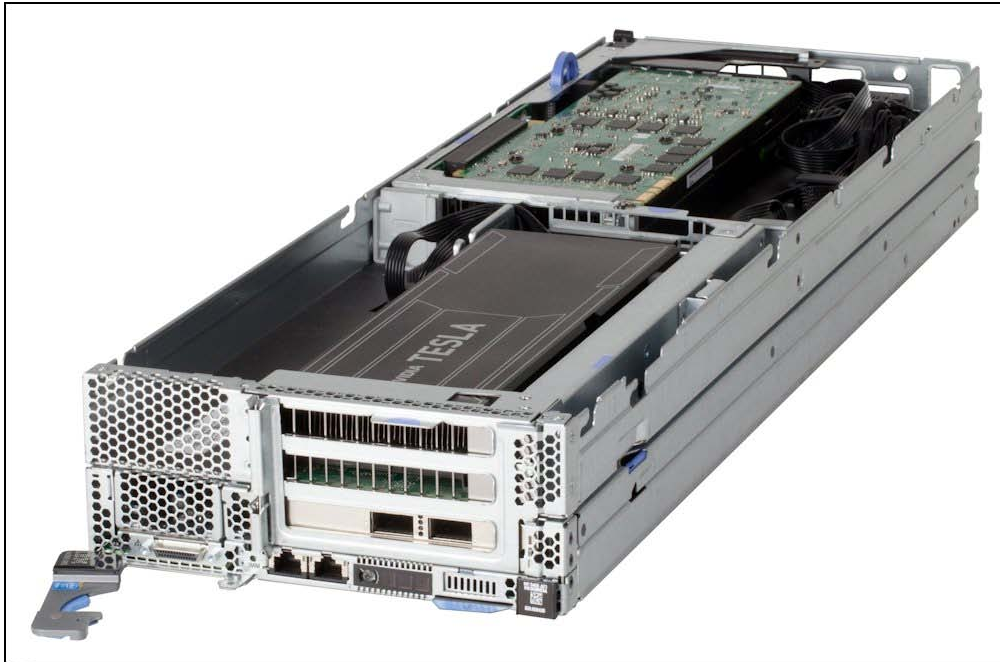
Figure 10. IBM NeXtScale PCIe Native Expansion Tray attached to an nx360 M5 compute node
