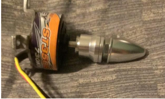
Figure 35 - Component, HobbyKing Donkey ST3508 730KV Brushless DC Motor
