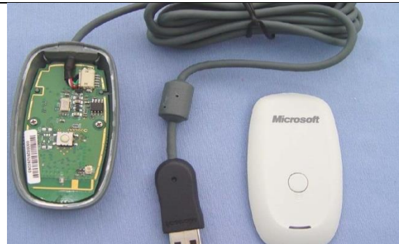
Figure 30 - Component, Xbox 360 Wireless Receiver
