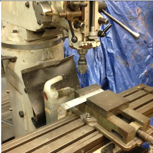
E 3 - Photo Album, Drilling Aluminum Mounting Bars
