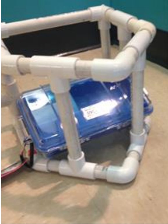
Figure 58 - Prototype Frame with Loose Housing
