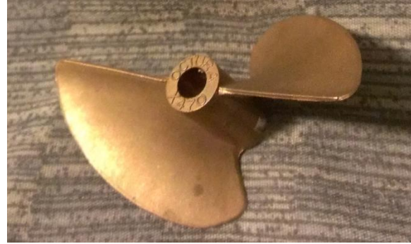
Figure 36 - Component, Octura X470 1.4 Dia. Beryllium Copper Propeller
