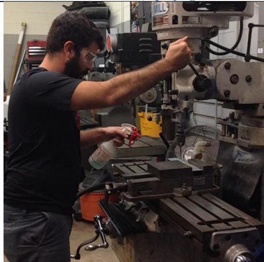
E 4 - Photo Album, Drilling Aluminum Mounting Bars 2
