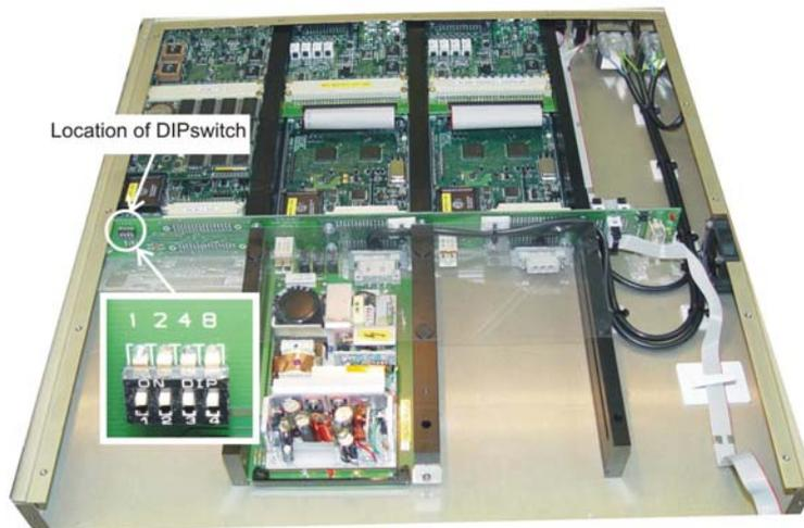
**Figure 3 - Open Flexi Box showing Chassis Number DIP Switches**
