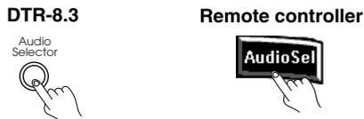
**Auto (automatic detection):** With this setting, the DTR-8.3 automatically detects whether the input signal is digital or analog. When a digital signal is not input, then the analog signal is played. This setting only appears if a digital input is selected for the Digital Input setting at Setup Menu → Input Setup Menu → Digital Setup Sub-menu (see page 49).
