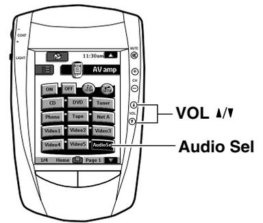
When using the remote controller, select AV Amp in the Home menu to display the operation menu.
