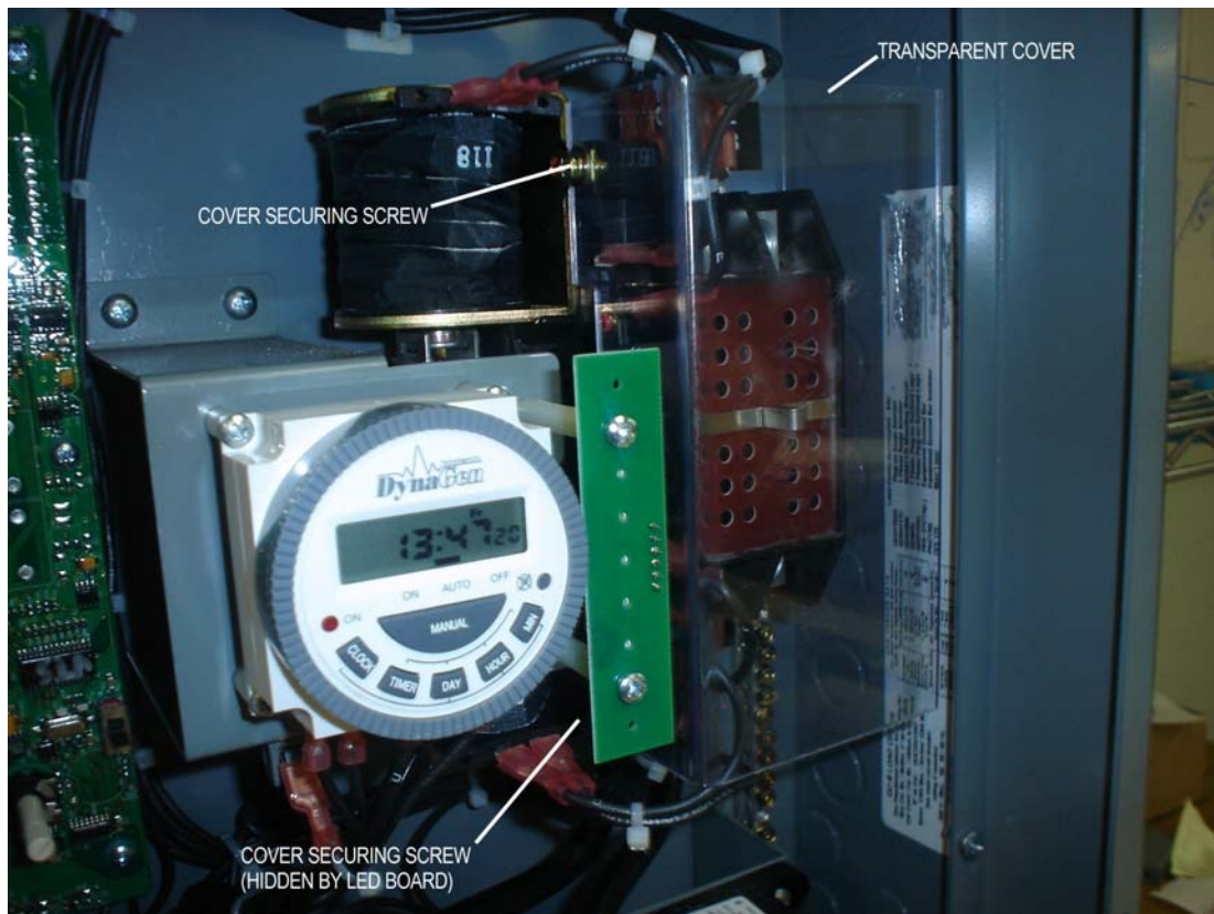
Figure 4. TRANSPARENT COVER SECURING SCREWS
