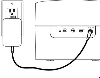
Attach AC adaptor cable to jack on back of the unit and plug the other end into a wall socket to play and charge iPhone/iPod.
