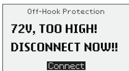
Figure 4.1 Over Voltage Warning
