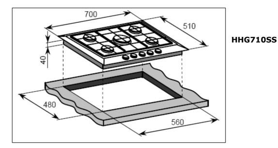
$\circ~$  Cut a hole in the worktop that corresponds with the relevant drawing above.
