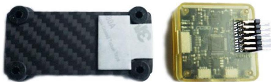
14.4 Paste the CC3D to the 3M tape on the controller board plate with the pins as shown below.
