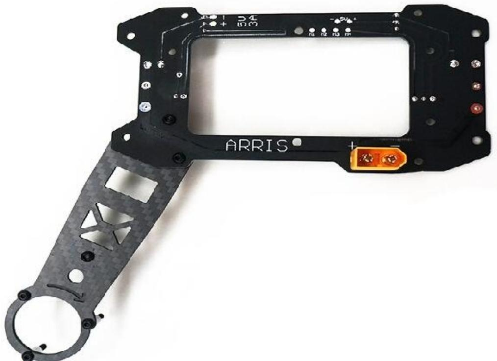
5.3 Install the remaining three arms to the PDB. NOTE: The etching on the arms should face up as in the photo below. For CC3D: the left front **motor rotation** is CW, the one next to it is CCW, and the one opposite to it is CW.
