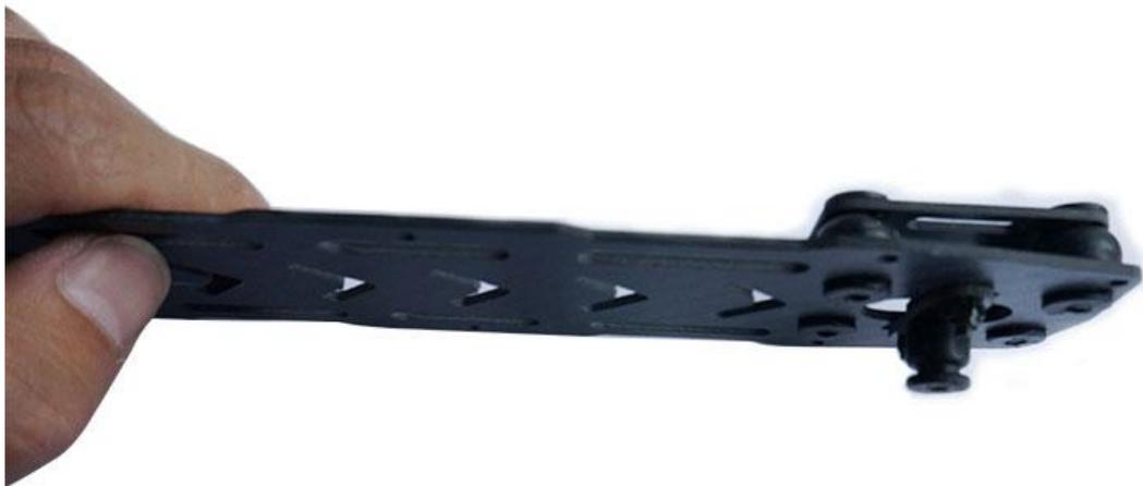
18. Connect the battery plate with assembled parts
