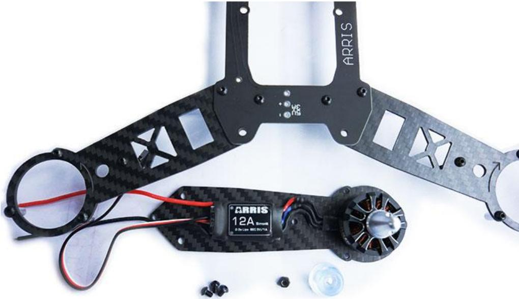
Pay attention to the motor and ESC wires. Tighten the nut with a socket wrench.
