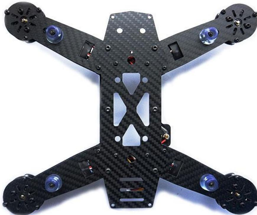
12. Install the aluminum standoffs using M3 x 8 screws.
