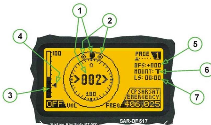
Fig. 3-4 Display Page 1 (360° Bearing Display)
