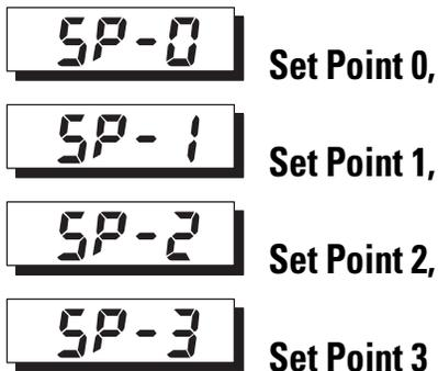
**Conditions of Use:** The Number of Multi-SP Uses parameter must be configured to either 1 or 2, and the Multi-SP Uses parameter must be configured to ON.
