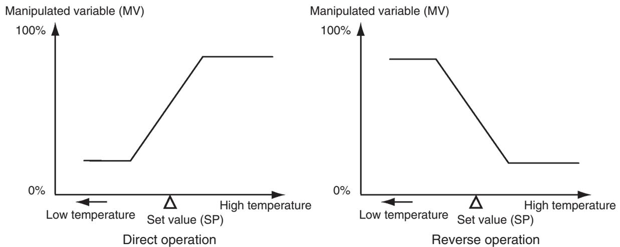
For example, when the process value (PV) temperature is lower than the set point (SP) temperature in a heating control system, the manipulated variable (OUT1) increases (ON) by the difference between the PV and SP values.
