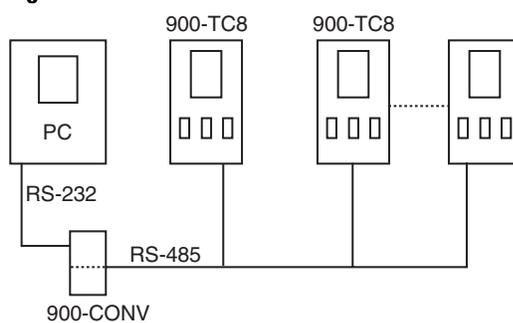
**Note:** The PC must have 900Builder software installed to configure/monitor the Bulletin 900-TC8.
