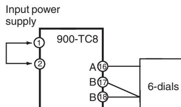
When calibrating a platinum resistance thermometer use wires of the same thickness as those used to connect the Bulletin 900-TC8.
