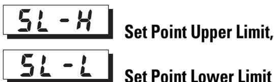
**Function:** These parameters allow you to configure the maximum allowable range for an operator to enter the set point value. The SP can be configured within the range defined by the upper and lower limit values in the Set Point Upper Limit and Set Point Lower Limit parameters. If an attempt is made to enter a SP value outside the upper or lower limit from the keypad the set point display will flash at the configured maximum upper- or lower-limit value.
