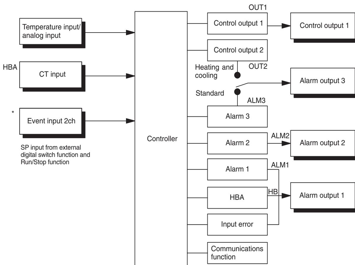
The Bulletin 900-TC8 temperature controller allows the user to carry out the following:
