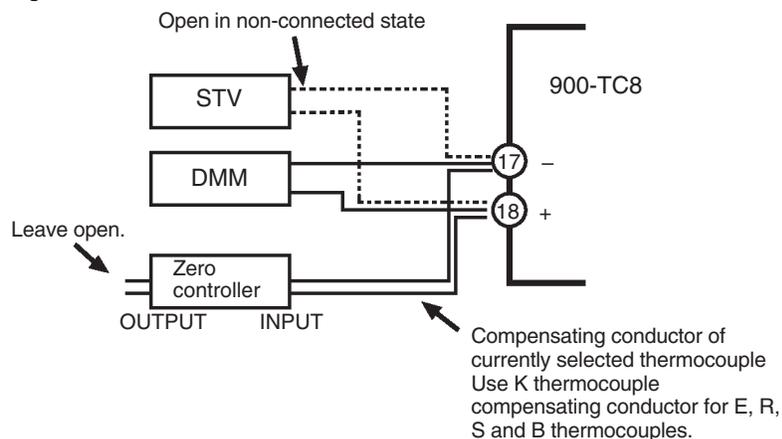
Disconnect the STV to enable the thermocouple of the cold junction compensator. When doing this, make sure to disconnect the wiring on the STV side.
