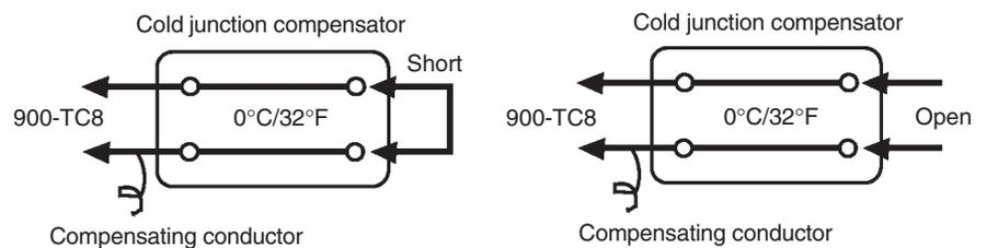
This example describes how to calibrate the Bulletin 900-TC8 when thermocouple input is currently selected on a Bulletin 900-TC8 supporting a thermocouple temperature sensor.
