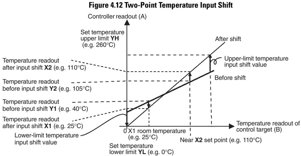
– **Equation 1:** Use the following equation to calculate the lower-limit temperature input shift value.
