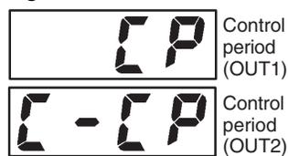
A shorter period may provide better ON/OFF control performance, we recommend setting the control period to 20 seconds or more. In the case of electromechanical relay outputs, doing this will improve its life expectancy. If necessary, readjust the Control Period by trial operation to meet the needs of your application.
