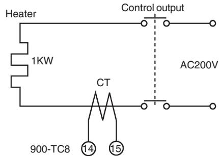
$$\text{Current during normal operation} = \frac{1000}{200} = 5 \text{ A} (< 10 \text{ A})$$
