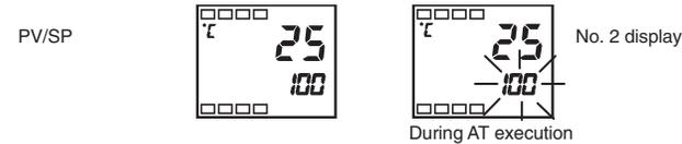
**Note:** Only the Communications Writing, RUN/STOP, and AT Execution/Cancel parameters can be changed during AT execution. Other parameters cannot be changed.
