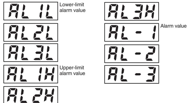
Alarm values are indicated by **X** in Table 3.H. When the upper and lower limit values are set independently, H is displayed for the upper limit value, and L is displayed for the lower limit value.
