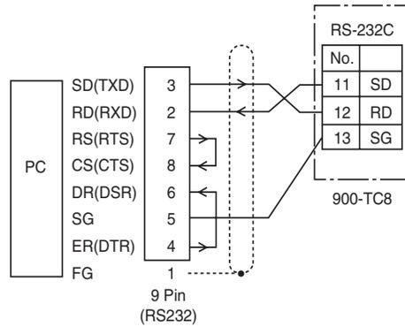
The RS-232C connection is one-to-one (PC to one Bulletin 900-TC8). The maximum cable length for RS-232 is 15 m. An optional 3 m RS-232C interface cable (Cat. No. 900-CP1x) is available as an extension cable if necessary. If you make your own cable, use shielded, twisted pair cable (AWG 28 or larger).
