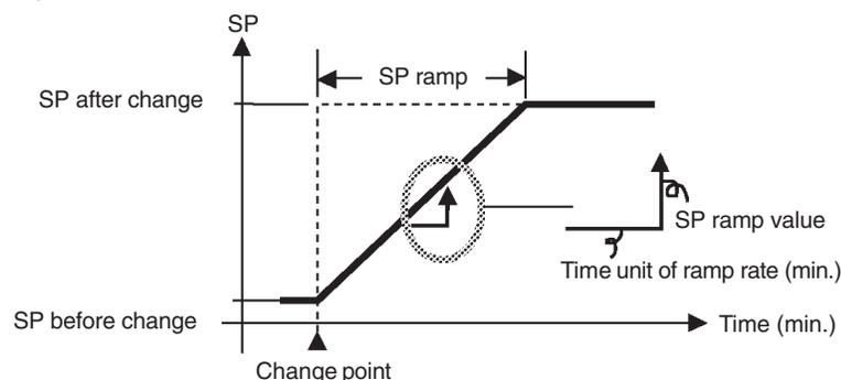
The maximum allowed rate of change during SP ramp is specified by the SP Ramp Set Value parameter. **Note:** The SP Ramp Set Value default is OFF, and the SP ramp function is disabled.
