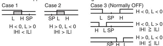
❺ Set value: 5 upper- and lower-limit alarm with standby sequence
