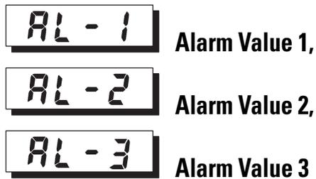
**Conditions of Use:** The alarm type must be set to either no alarm or a setting other than upper and lower limit alarm. The control mode must be set to standard control (Alarm Value 3).
