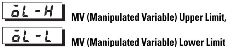
**Conditions of Use:** The control method must be 2-PID control, and the ST parameter must be set to OFF.
