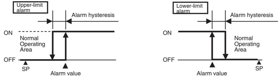
Alarm hysteresis is independently set for each alarm output in the alarm Hysteresis 1 to 3 parameters (Advanced Setting function group). **Note:** The default is 0.2 (°C or °F depending on your units selection).
