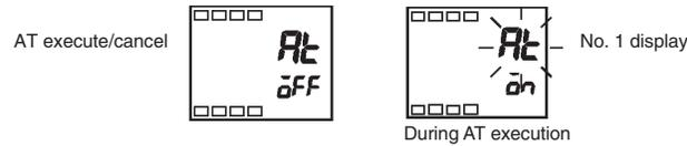
If you move to the Operation function group during AT execution, the No. 2 display blinks to indicate that AT is being executed.
