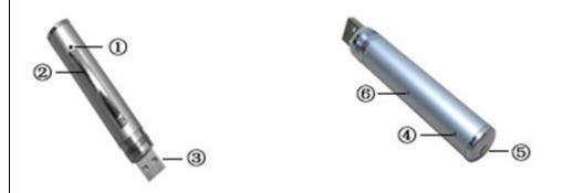
①Camera ②MIC ③USB ④Record and Power Light ⑤Power ON/OFF ⑥Reset
