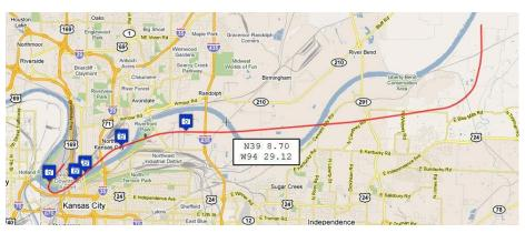
This map shows the full sortie track and all of the photo locations. (This is a a simplified example with only five photos and an abbreviated GPS track.) The Sortie Overview map is invoked by clicking the "Map All" button to the lower right of the photo listing table.
