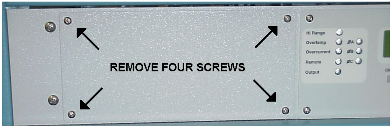
Figure 6-2: Current Limit board access panel
