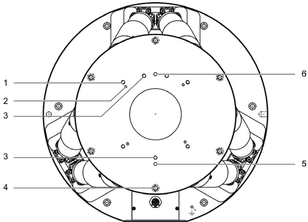
Figure 9: Mounting and locating holes in the moving platform
