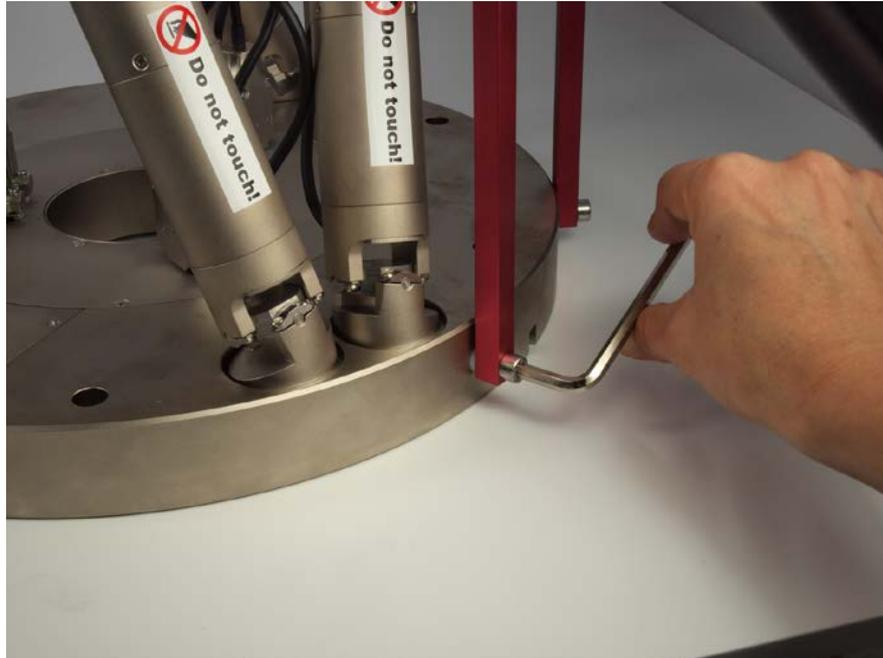
Figure 14: Transport lock on the base plate
