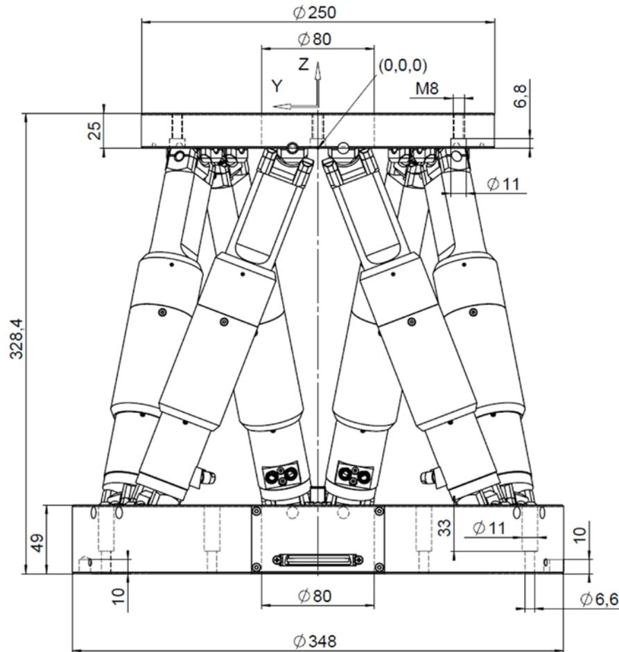
Figure 15: H-850 Hexapod front view (dimensions in mm)
