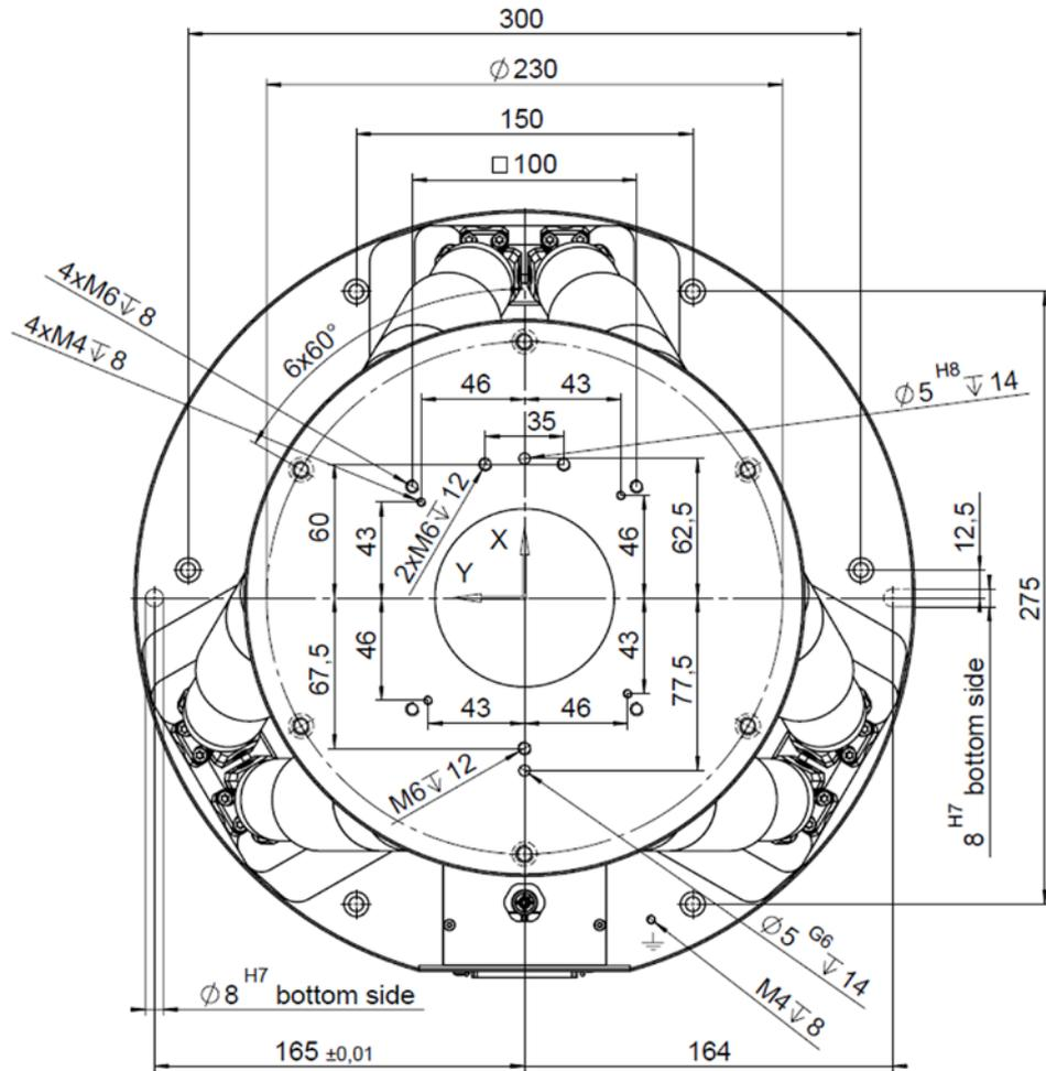
Figure 16: H-850 Hexapod top view (dimensions in mm)
