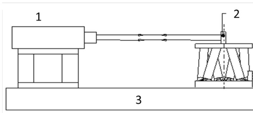
Figure 19: Test setup for measuring the X or Y axis.
