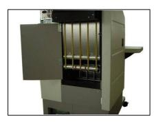
Open the rear cover of the device (chapter 4.4). Inside the device you will see five yellow belts, which are driven by six drive sprockets. The outer belts can be shifted to the middle for the processing of smaller formats. First familiarise yourself with the position of all 6 drive sprockets by following the path of the conveyor belts in the device. One of the sprockets can only be reached
