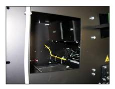
The cylindrical mirrors are accessible via the middle and lower service openings respectively. Carefully clean the mirrored surface using a cloth from the cleaning kit supplied with the scanner. For heavy soilage moisten the cloth with SCAMAX® Lens Cleaner. Any streaks that might be left can be removed using a dry cleaning cloth.
