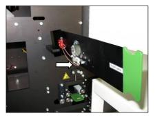
First pull the lamp bases out of the guide completely. Remove the dust. Avoid touching the lamp bodys with your bare hands. Before replacing the lamp bases, check that the halogen lamps are fitted correctly. Adjust the halogen lamps where appropriate, as described in Chapter 9.1 'Replacing the halogen lamps'.
