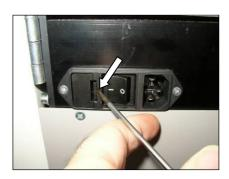
To check or replace the fuses use a small screwdriver to push the retaining latch to the left.
