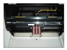
Next remove the light barrier support above the feed belts. To this end, loosen the knurled nuts and remove the proximity switch from the centring pins. Place the proximity switch as far to the right as is allowed by the connection cable.
