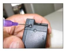
Attach the needle to the syringe with a screw action. Pull the plunger upwards till it reaches the 1 ml level.
