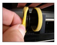
The worn rubber linings can simply be removed from the retaining rollers by pulling to the left.
