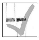
After you have mounted the lamp, check that it is fitted correctly. To do this, hold the lamp support horizontally in front of you and look directly at the newly mounted lamp. Focus on the lamp filament and its reflection. The two lamp filaments should be reflected in the concave mirror as shown in the illustration to the left. The filaments should be at the same level and should be spaced apart by 0.5 to 1 mm.
