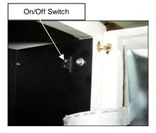
Open the display panel at the front of the scanner (refer to chapter 4.5). Use the switch located behind the display panel to turn the scanner ON. Close the display panel.
