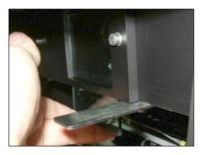
Slide the filter downwards to release it from the frame. Clean the filter using a lint-free cloth. If the filter is very dirty, moisten the lint-free cloth with SCAMAX® Lens Cleaner. Insert the glass in the frame and hold it there till the catch engages. Make sure not to touch any of the glass surfaces.
