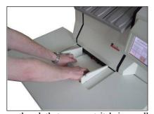
Select the **BATCH** mode on the display. The input hopper plate drops into its bottom position. Apply cleaning fluid to a lint-free cloth and press the **TRANSPORT** button. All belts and rollers will now run for a maximum of six minutes. Move the cloth forwards, above the sensor, and the input hopper plate will drive into its upper position. Retain a firm grip
