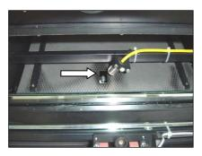
The ultrasound double feed detector is located right behind the feeder. It can be set to ACTIVE or INACTIVE via the menu. (for detailed description refer to chapter 5.4).
