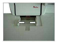
The paper guide extensions are divided. To make it easier to insert single sheets manually, the upper section of the guides can be removed. Loosen the handscrews and remove the upper part of the guides.
