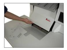
Set the paper guides to their widest opening and remove the top parts of the guides (see chapter 3.1). Next, remove the weights of paper input if fitted. Remove the front cover as detailed in chapter 4.1.
