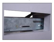
The interface connection is located on the back of the scanner at the bottom. The connection consists of a 68-pin SCSI connector and a 9-pin Serial connector, which is used as service interface, a footswitch connection or adapter connection if two footswitches are being used.
