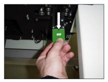
You will recognise the paper guide bar by its green marking. The bar is held in position by a centring pin and centring screw.
