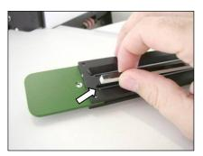
The smaller of the two slots at the bottom side of the paper guide bar is fitted with spring-loaded bolts. Push the metal bar into the slot till it clicks in, making sure the black side points outwards. Re-insert the paper guide bar into the scanner (see chapter 8.1).
