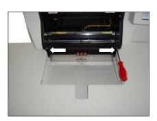
First unscrew the two Phillips screws on the feed device. You can now remove the cover plate carefully.
