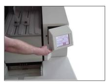
To open the housing, grip the bottom lefthand corner and swing the housing towards the right.
