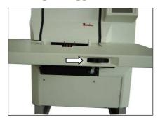
By rotating the adjustment wheel on the front side of the table, the spacing of the lateral guides of the document feed can be adjusted to the width of your documents. The width of the widest document should be selected for documents with mixed formats.
