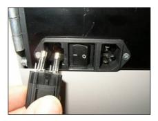
Remove both fuses and replace with new ones of the same type (fuse type T6.3 A 250V).
