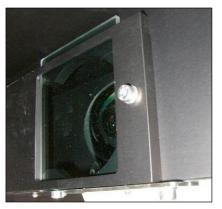
The front side of the condenser lens facing the lamp can be reached through the front opening (chapter 4.1) when the lamp support is pulled out. Now clean the front side of the condenser lens. In order to clean the rear side of the lens facing away from the lamp, the infrared filter glass (i.e. the glass plate in front of the lens) must be removed.
