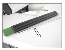
The white scan background is a metal bar, which is located directly beneath the storage rack of the weights for paper input (see chapter 3.3). It has to be inserted into the paper guide bar. Remove the paper guide bar as detailed in chapter 8.1 and insert the bar.
