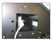
The upper front lens and deflection mirror are accessible via the upper square service opening and the opening behind the front cover.
