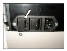
The fuses of the SCAMAX® scanner are located inside the power supply unit at the rear of the scanner, immediately left to the power switch.
