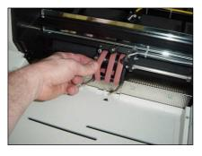
Pull the existing belts off the rollers by moving them to the left hand side. Slightly tilt the belt assembly while pulling to aid removal of the belts over the stop.
