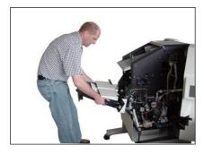
Pull the table away from the device carefully, without tilting. Take care that the paper guide plate, which projects into the device, is not damaged or bent. Hold the table in the manner illustrated in the diagram opposite. Place the table in a protected position.
