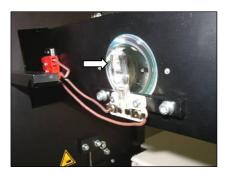
Pull the lamp base completely out of the device.
