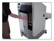
To open the rear cover turn the lock a quarter of a turn anti-clockwise and pull the cover open.
