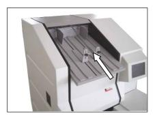
Adjust the front stop to accommodate the longest documents to be scanned. The height of the exit deflector can be adjusted by changing the height of the horizontal bar on the front stop. Loosen the knurled nuts and move the bar up or down, then fasten the nuts.
