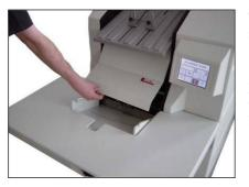
The front cover is held in position by magnets. To remove it, first engage auto feed as described in chapter 5.2/5.2.1, to drive the input hopper plate downwards. Grip the bottom edge of the cover and pull it towards you.
