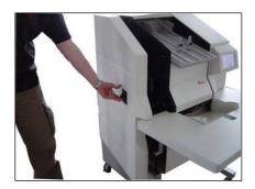
The left side cover can be opened just like a car door. Pull the black handle slightly upwards and swing the side cover towards the back. Behind the cover are the service openings for cleaning and accessing the scanner.
