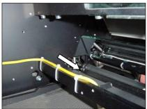
It takes a little practice to replace the paper guide bar. Hold the bar so that the marking "TOP" faces upwards. Then insert it into the device, keeping it as level as possible.
