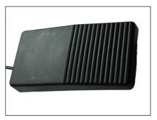
For example, the paper separation can be activated / deactivated via the foot switch. This is particularly useful when difficult documents (folded, stapled or very thick ones) are to be processed and the operator needs both hands to accomplish the task. As long as the foot switch is pressed the paper separation is off, the seperator rollers are lowered allowing the transport of documents approaching maximum
