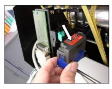
To insert a cartridge, gently push it into place from the right and lock it by pressing the green lever down until it clicks into position.
