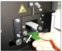
Lock the bar in its final position by placing the centring hole in the handle of the paper guiding bar over the corresponding centring pin on the left side of the device.
