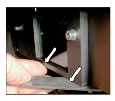
The infrared filter glass is held in its mounting by a locking device. Swivel the locking device to the side. At the same time, hold the infrared filter glass firmly so that it can not slip downwards out of its mounting after the locking device has been released.
