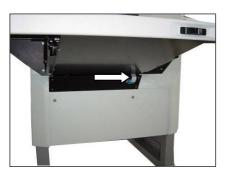
Remove the cable plug connection beneath the table.
