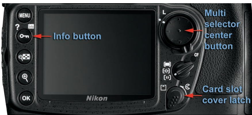
FIG 6 – D300 control differences
