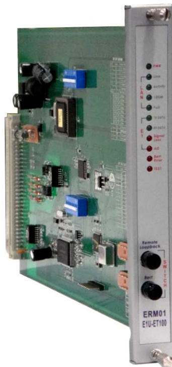
Figure 1-1 : Physical outlook of the E1U-ET100 line card.
