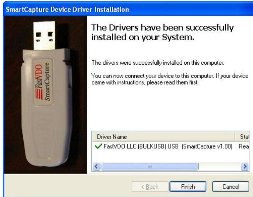
Click Finish to complete the Driver installation and plug in the device.
