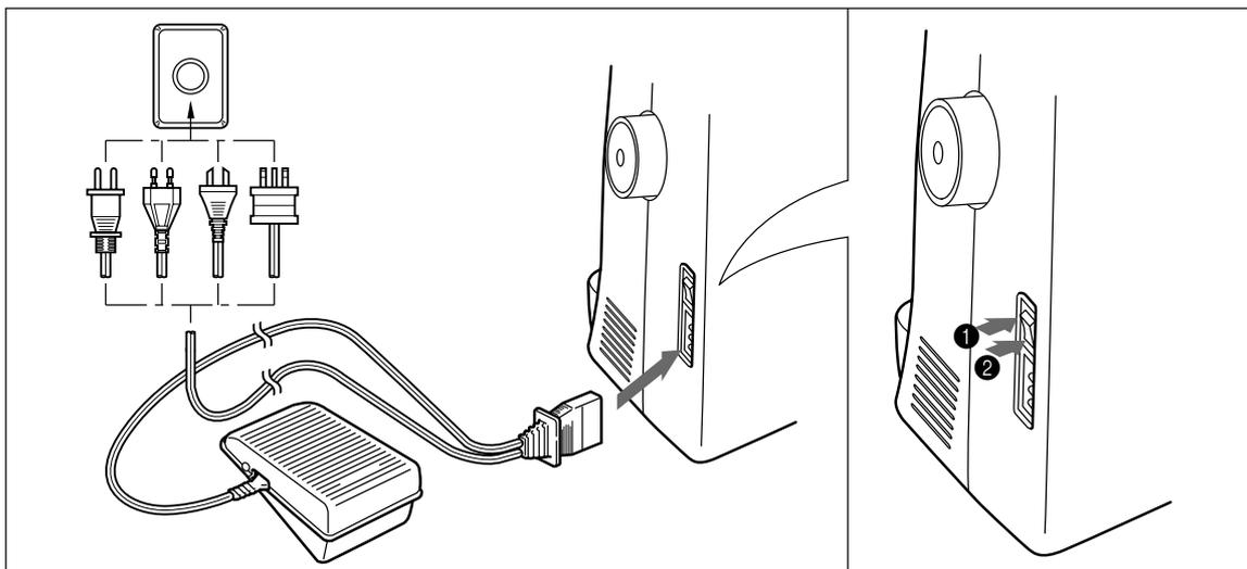
1. Connect the three-prong plug into the machine.
