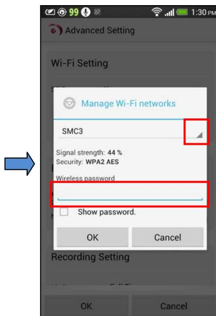
Click on the arrow button to select the Wireless router, and then type the password. Click on **[OK]** button to save the settings.
