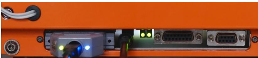
(left-to-right direction. UC100 device LED 1 and LED 2, control board LED 1 and LED 2)
