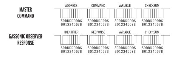
To allow the Gassonic Observer to distinguish between the address field and other fields, D7 is always set in the address field and always cleared in other fields.
