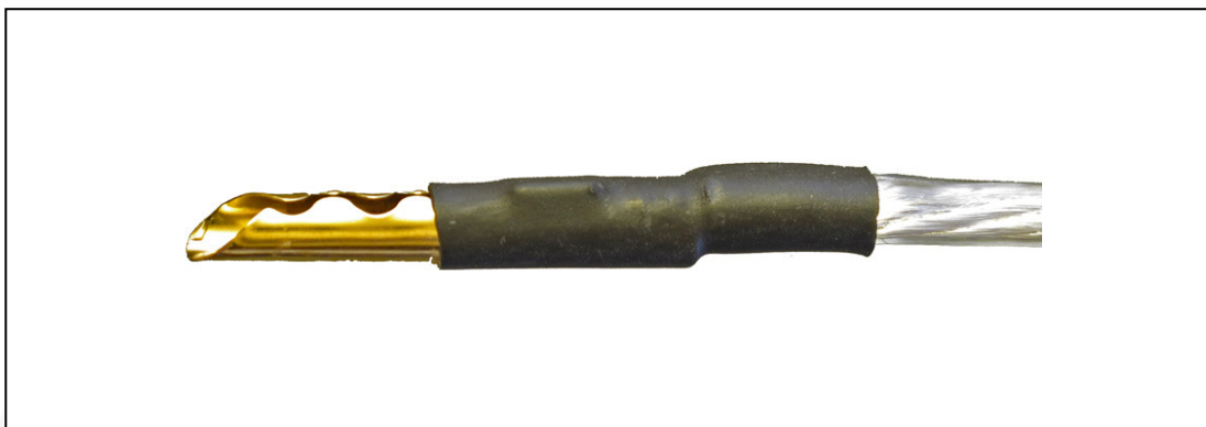
Figure 8. Recommended Loudspeaker Cable Termination
