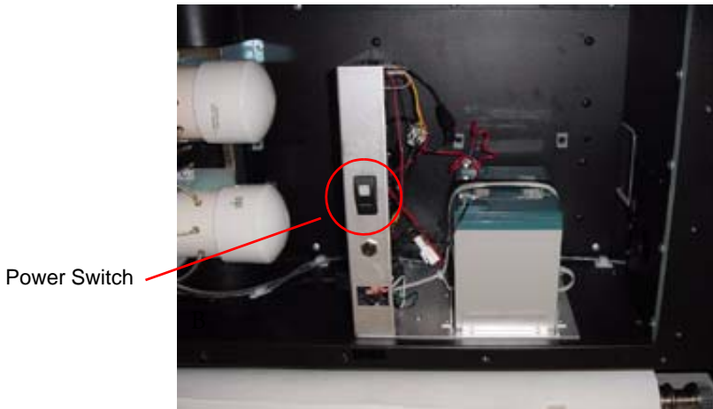
Figure 1-3 Battery Back-up Option
