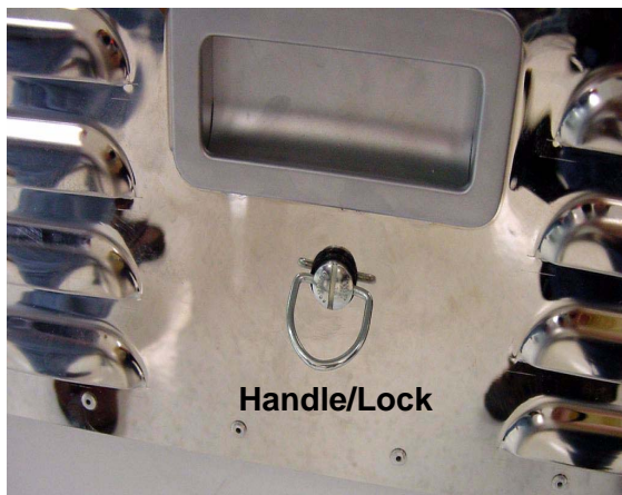
Figure 3-19 Paper-Feed Access Door Lock and Handle
