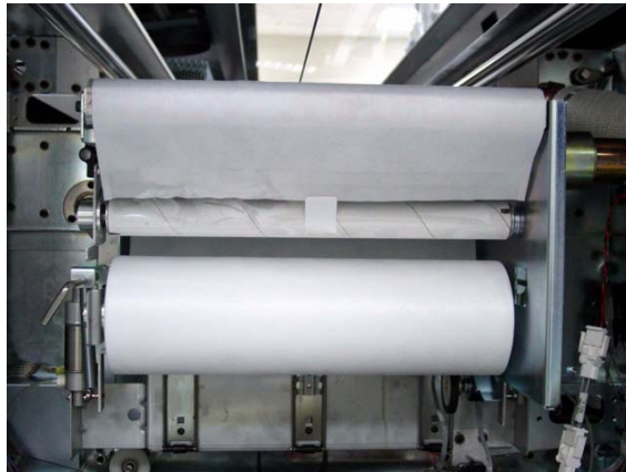
Figure 5-15 Attach the Cloth to the Take-up Core
