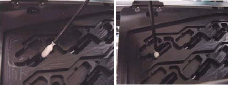
Figure 5-6 Cleaning the Drain Slots and Drain Holes
