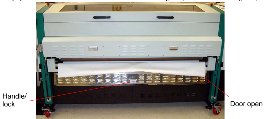
Figure 3-18 Open Paper-Feed Access Door
