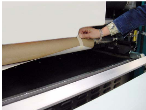
Figure 3-13 Align and Tape the Media
