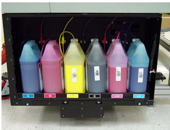
Figure 2-1 Ink Tray (1-Gallon Bottles Shown)
