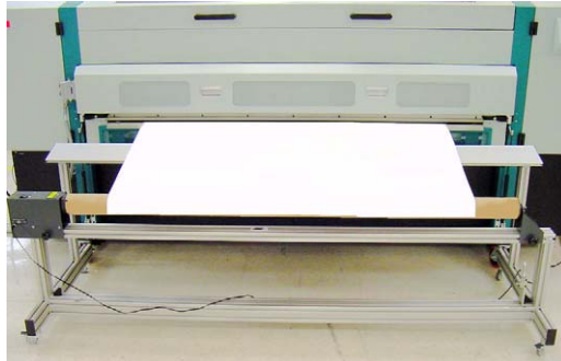
Figure 3-22 Attaching Media to the EMTU Core
