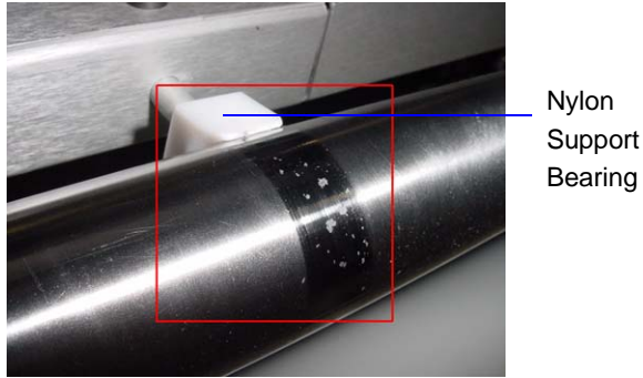
Figure 5-2 Take-up and Supply Dancer Bar and Nylon Support Bearing
