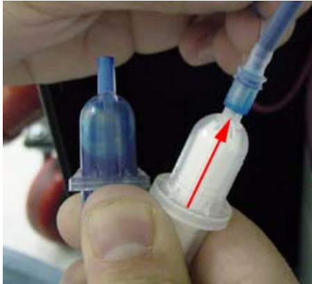
Figure 2-6 Attach Tube to the New Filter
