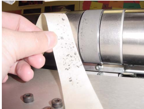
Figure 5-3 Press Fresh Tape on the Encoder Wheel
