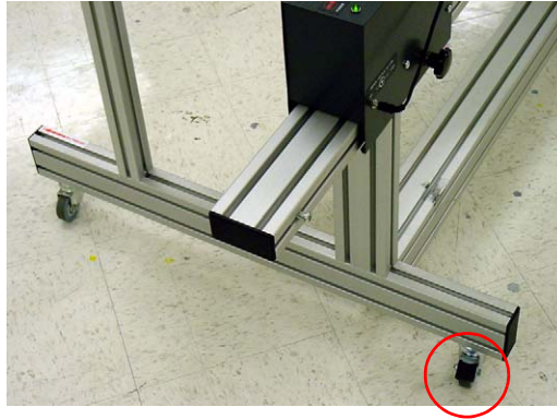
Figure 3-21 Correct Position of the Left Side of the EMTU
