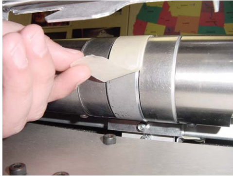
Figure 5-3 Press Fresh Tape on the Encoder Wheel
