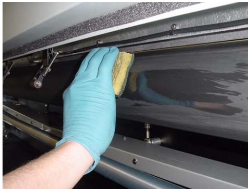
Figure 5-1 Cleaning the Media Drive Roller
