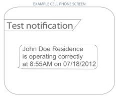
Important: Test your Pit Sensors by submerging them into a cup of water. This will trigger the unit to sound an audible alarm and send a text notification to all phone numbers programmed into the unit. Test the battery backup system by unplugging the A/C power adapter from the unit. All phone numbers programmed into the unit will receive the text notification.
