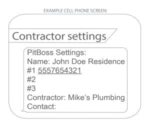
(Optional Contractor Setup)- To configure the contractor's contact phone number, text the unit using the following format: Contact{space} 888-454-5051.
