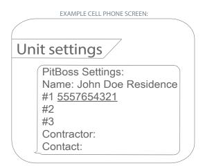
(Optional Contractor Setup)- Your PitBoss allows you to configure a contractor name with associated contact information. When this information is configured, the PitBoss appends this contact information to the end of alarm notifications (input alarms, low battery, power loss, etc.) so you know who to call in an emergency. To configure the contractor name, text the unit using the following format: Contractor{space} Mike's Plumbing.
