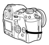
Power ON : Set the power switch to ON.
