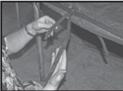
19- Using the longer piece of strapping sewn to the mesh, wrap it down, under, and around the top rail until it comes back out. (See steps 20, 21, & drawing "A")
