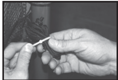
24- Bundle the loose ends of the Enclosure Cinch-Cord together and secure with plastic tie. Warning - failure to do this step may result in serious injury, strangulation or death.
