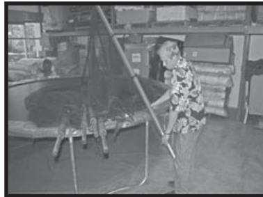
14- Select one enclosure pole and align holes on lower section with holes on one leg extension (extension with 2 holes)
