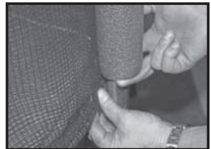
18- Slide enclosure pole foam up and work mesh drawstring down between enclosure pole and top rail so that drawstring is below top rail around the perimeter of trampoline.
