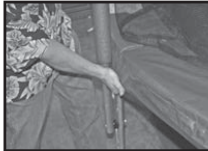
17- Firmly pull down pad cover edging so that padding completely covers top rail. Pull down into place.
