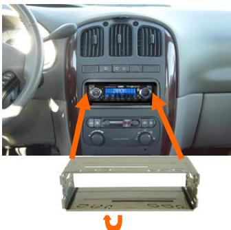
**NOTE:** Before installing the unit, please remove the two screws.
