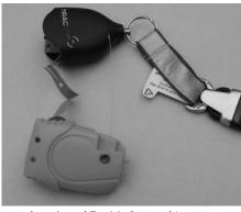
A correctly activated TracMe Personal Locator Beacon. In this state, it transmits the "Help....Emergency" voice message.
