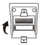
5. Then install screw back to end procedure.
