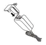
Please plug in power adaptor to wall power socket will light in a power Indicator. Then plug in another power adaptor terminal to S1 main board will light in a Indicator on main board.
