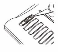
3. Then install button casing back on the main board.
