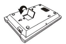
3. According to system configuration to set DIP switch by clamp.
