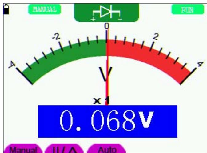
figure 19: Diode Measurement
