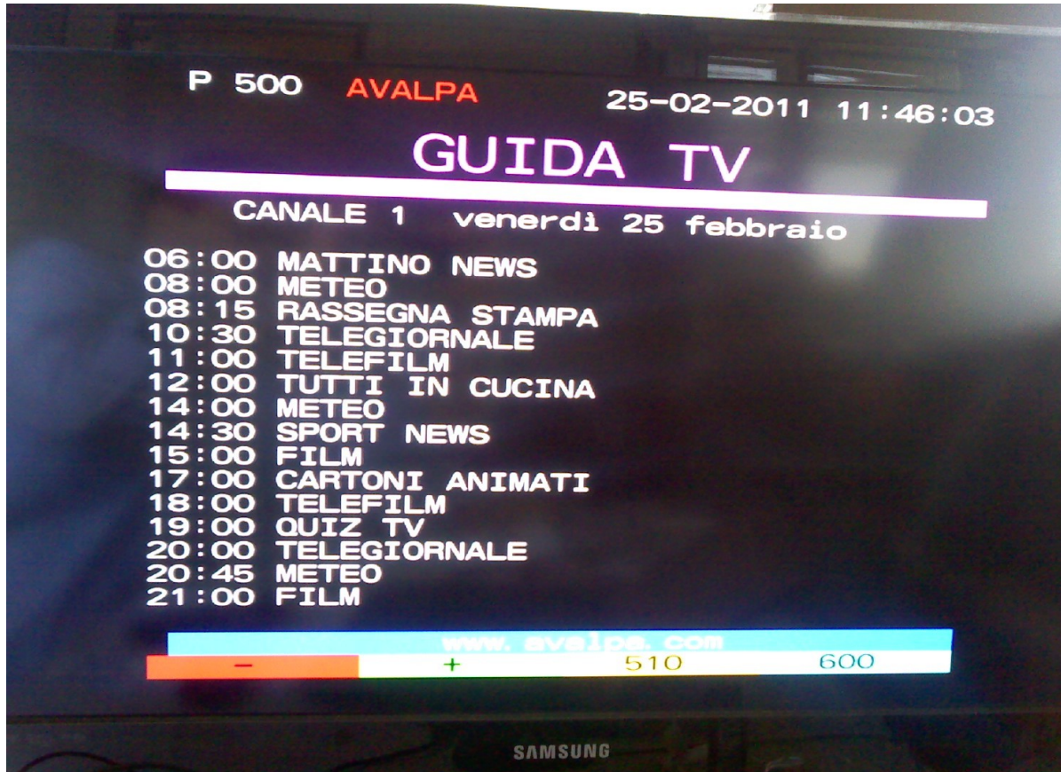
Figure 18: Example of EPG data inserted into teletext
