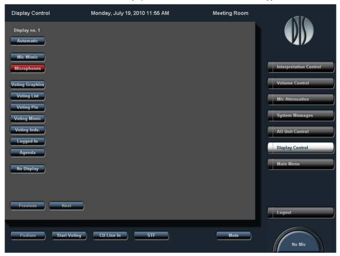
The screen will show a button menu for all the CDA displays, which are configured in the CAA in Setup/Equipment/CDA Displays'. Up to 8 displays can be used.
