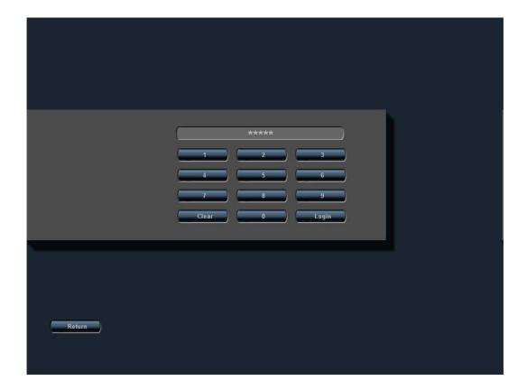
The users must enter their numeric code and press [Login]. Mistakes made when entering the code can be erased by pressing [Clear]. There is no limit to how many times the users can retry to enter their code.
