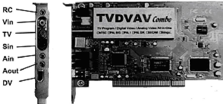
**RC** : For remote controller IR receiver(bundled in package) input
