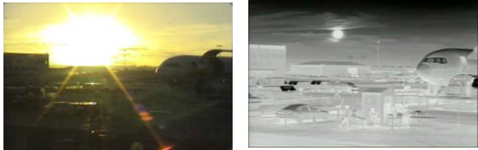
Figure 2-4: Images facing sun from standard camera (left) and thermal camera (right)
