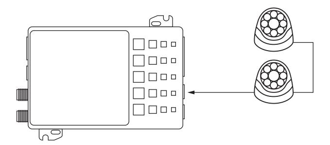
Connect the Camera ONE (the hub camera please checks the cameras and you will find a sticker of Hub camera) connects directly to the J204 port of vigilant. Connect the Camera Two with the camera One and connect the camera three with camera 3 and so on. You can set the camera number by using the following configuration equipment.
