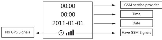
3. It will display as following after receiving GPS signal from more than 4 satellites: " T shows it can position.
