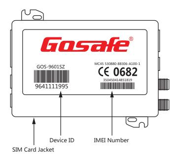
**IMEI:** Sticker on the bottom of the unit mentioned the IMEI number of the Modem used in the device.
