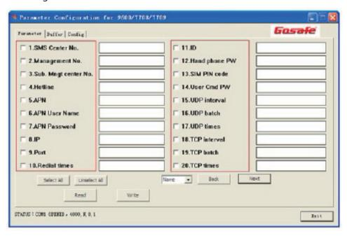
1. Fill in the APN, IP address, Port, Redial time, SMS center no., Management no. and Sub management no...
