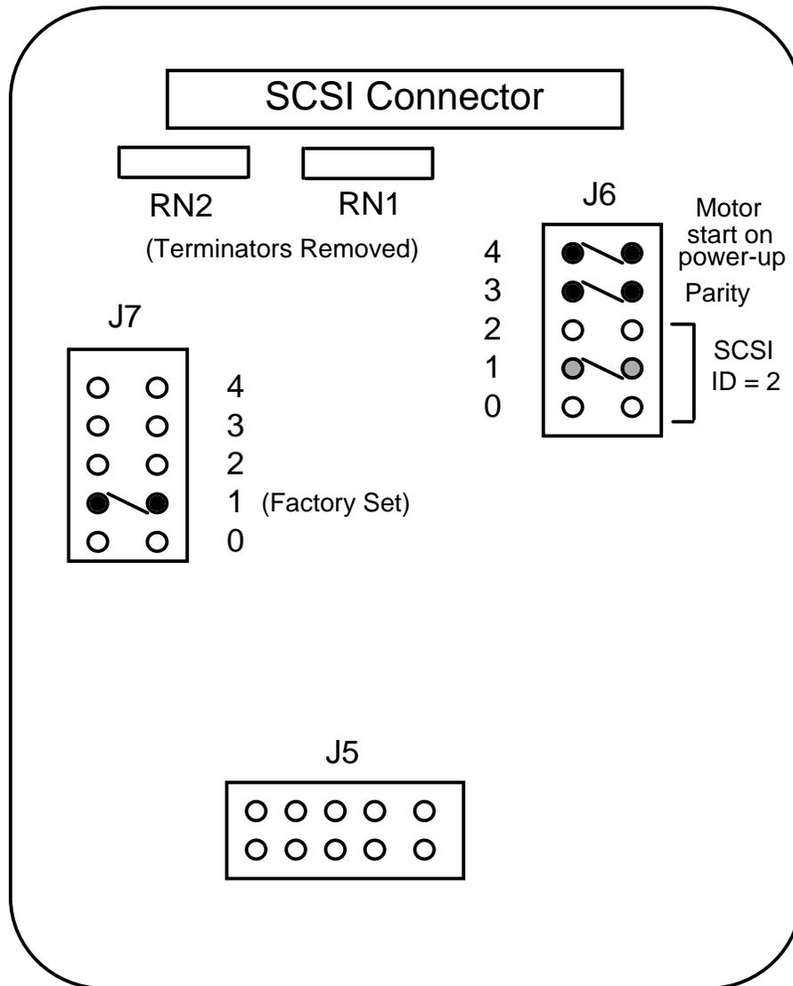
Figure B.6 - Maxtor MXT-1240S Hard Disk
