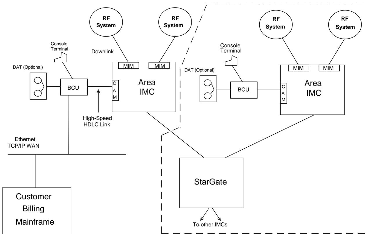
The dotted lines enclose one optional setup for a StarGate (multi-node) billing architecture.
