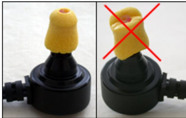
Figure 2.8: A correctly squeezed foam eartip (left), and an incorrectly squeezed foam eartip (right).
