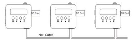
The function of the two in-phase signal port appears the same, general net cable can be used as the connection cable, in a single network, only one controller works at the Master style sending in-phase data signals, while other controllers work at the Slave Style receiving in-phase data signals.
