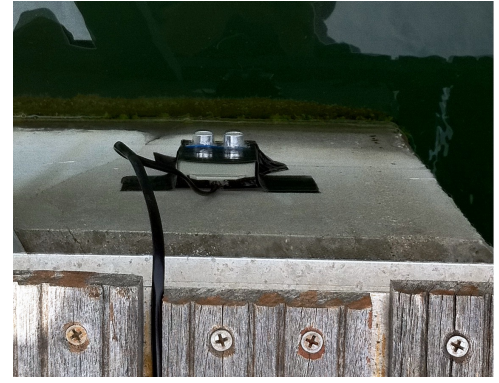
Fig. 6. Berth sensor mounted on the pontoon forefront as seen from above
