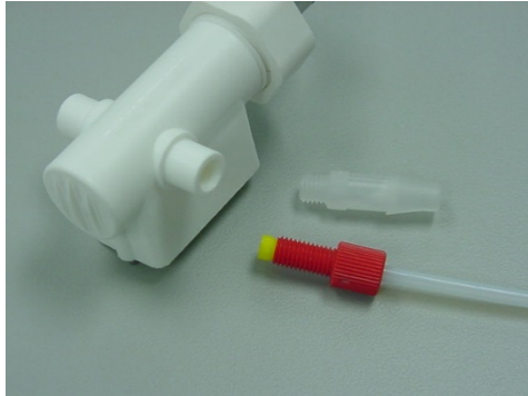
Example of ¼-28 UNF bottom sealing fitting (bottom) and face sealing fitting (top)
