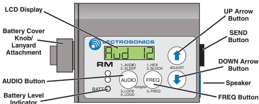
The RM gives you remote control of SM Series transmitters using an audible tone delivered to the transmitter's microphone. When the SEND button is pressed, a "dweedle" tone will play from the RM speaker and the parameter on the transmitter will be set immediately. The transmitter must be configured to accept commands from the RM (see page 6). Adjustments can be made to set:
